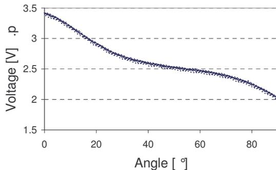
Fig. 8. PIP angular sensor measured characteristic.
