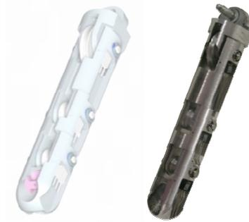
Fig. 5 CAD drawing and prototype of the *fully underactuated* finger (ring).
