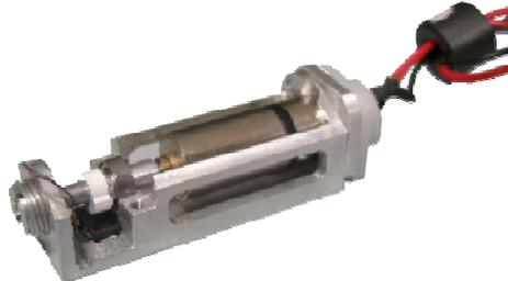
Fig. 9. The proximity sensor for detecting angular position
