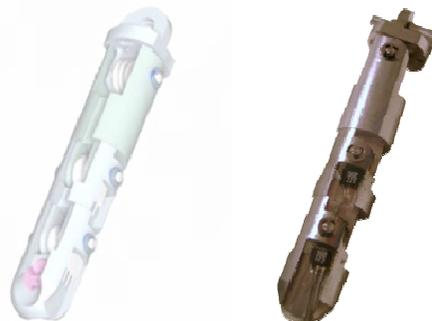
Fig. 4 CAD drawing and prototype of the *hybrid actuated* finger (index).
