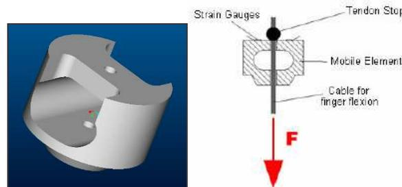
Fig. 11. Cable tension sensor: working principle.
