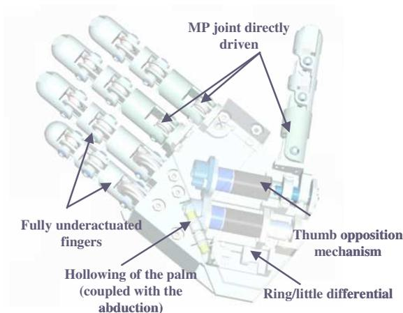
Fig. 2 The CAD drawing of the *iCub* Hand.
