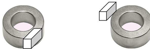
**Figure 14:** An hall sensor is placed at the edge of a large magnet, magnetized across the diameter. The sensor can be placed frontally (left) or laterally (right).
