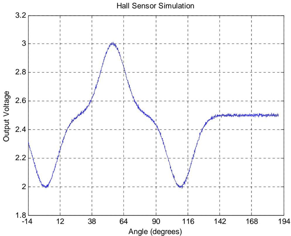
**Figure 8:** Simulation of the hall sensor response in the conditions of test with bigger magnets.
