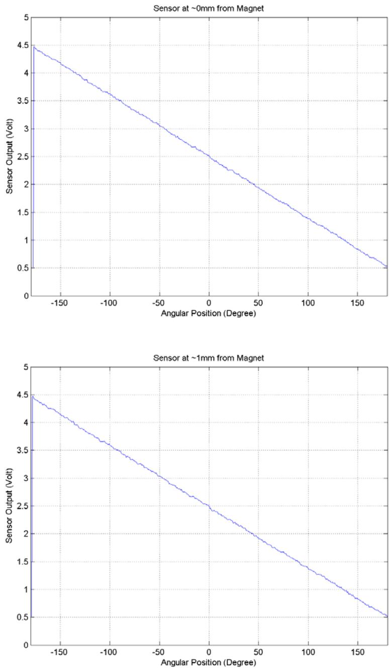
**Figure 21.** Magnitude of sensor output as a function of angular position. Cases where the magnet and sensor are at close proximity.
