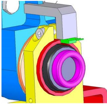
**Figure 15.** Hall sensor and ring magnet. Mechanical assembly.
