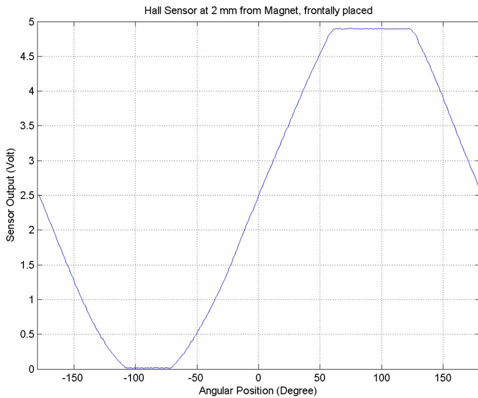
**Figure 16.** Frontally placed sensor. Output as function of magnet rotation. Notice saturation when sensor is placed at 2mm from the magnet.
