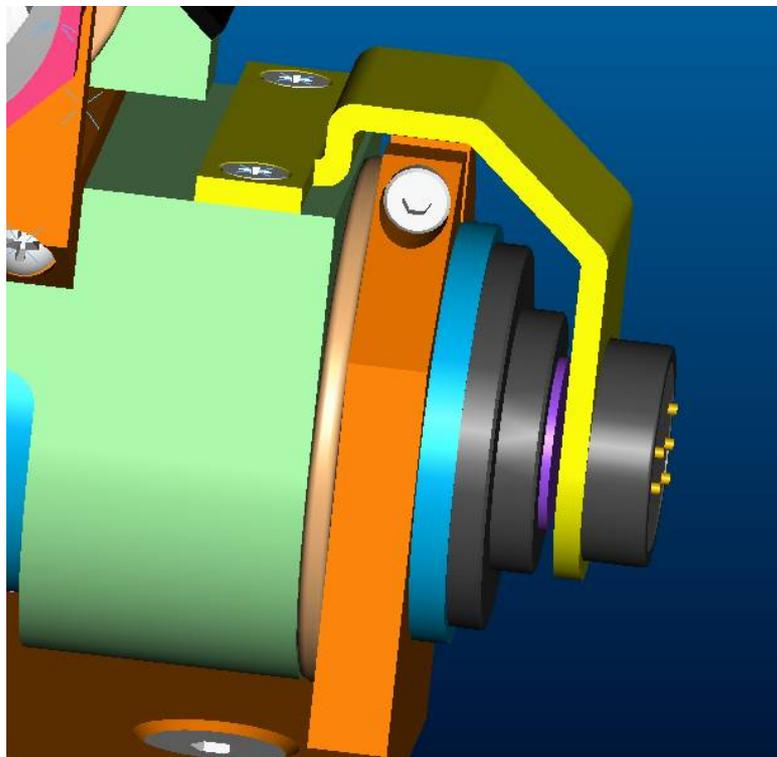
**Figure 20.** Mechanical assembly of the GMW360ASM and ultra-thin magnet in the iCub head.
