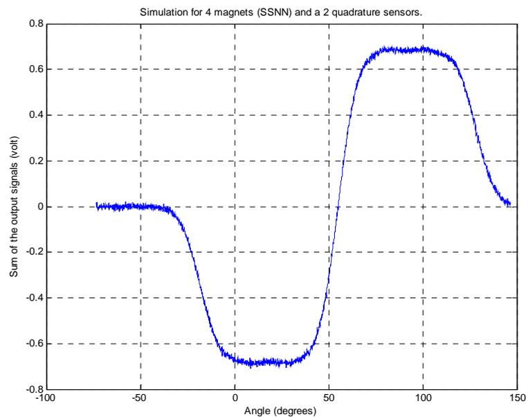
**Figure 12:** Sum of the response of 2 sensor/4 magnet configuration.
