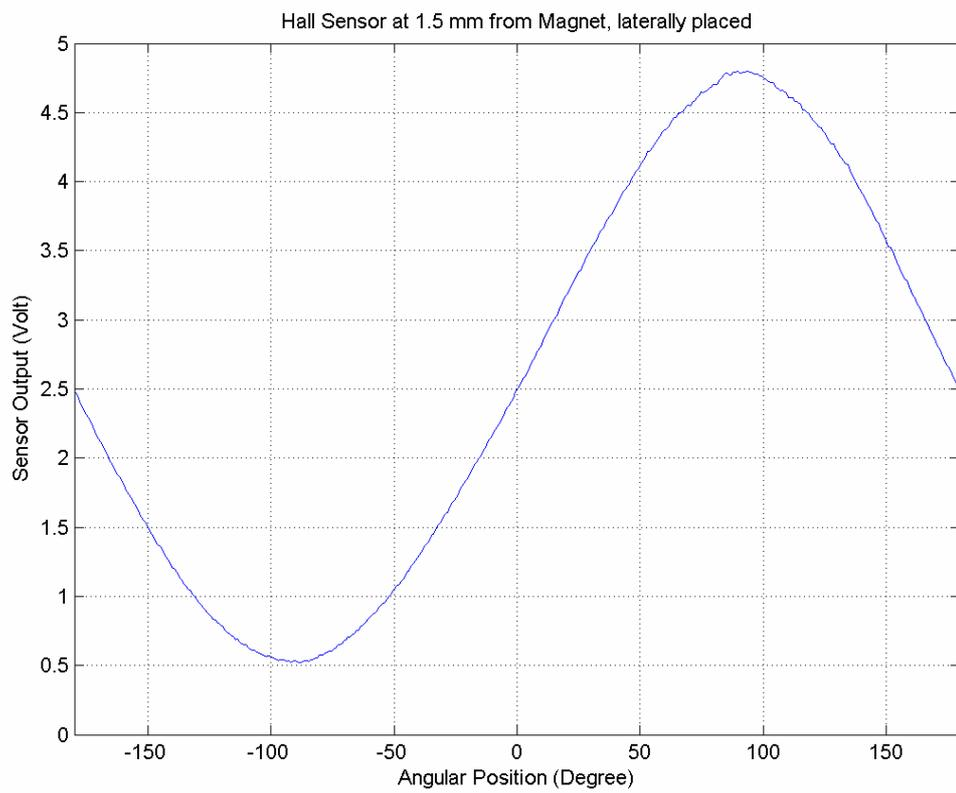
**Figure 17.** Laterally placed sensor. Output as a function of magnet rotation.
