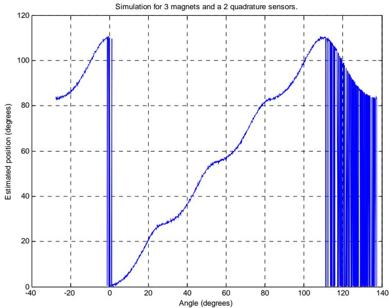
**Figure 11:** Simulation for absolute positioning response of 2 sensor/3 magnet configuration.
