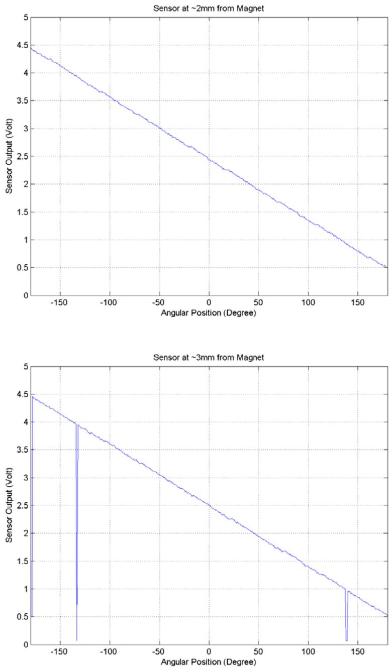
**Figure 22.** Magnitude of sensor output as a function of angular position. Magnet and sensor are separated apart about 2mm and 3mm.
