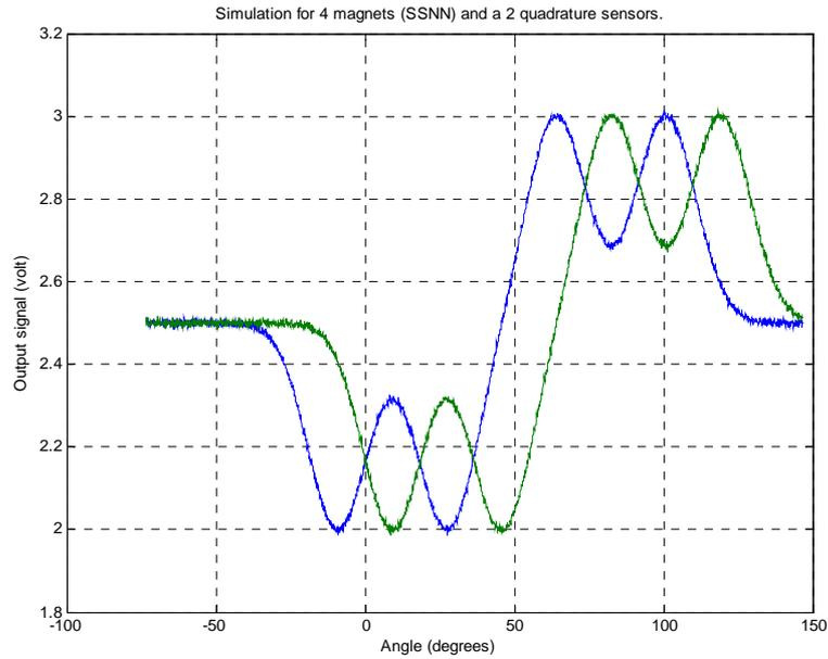
**Figure 13:** Simulation of the response of 2 sensor/4 magnet configuration.
