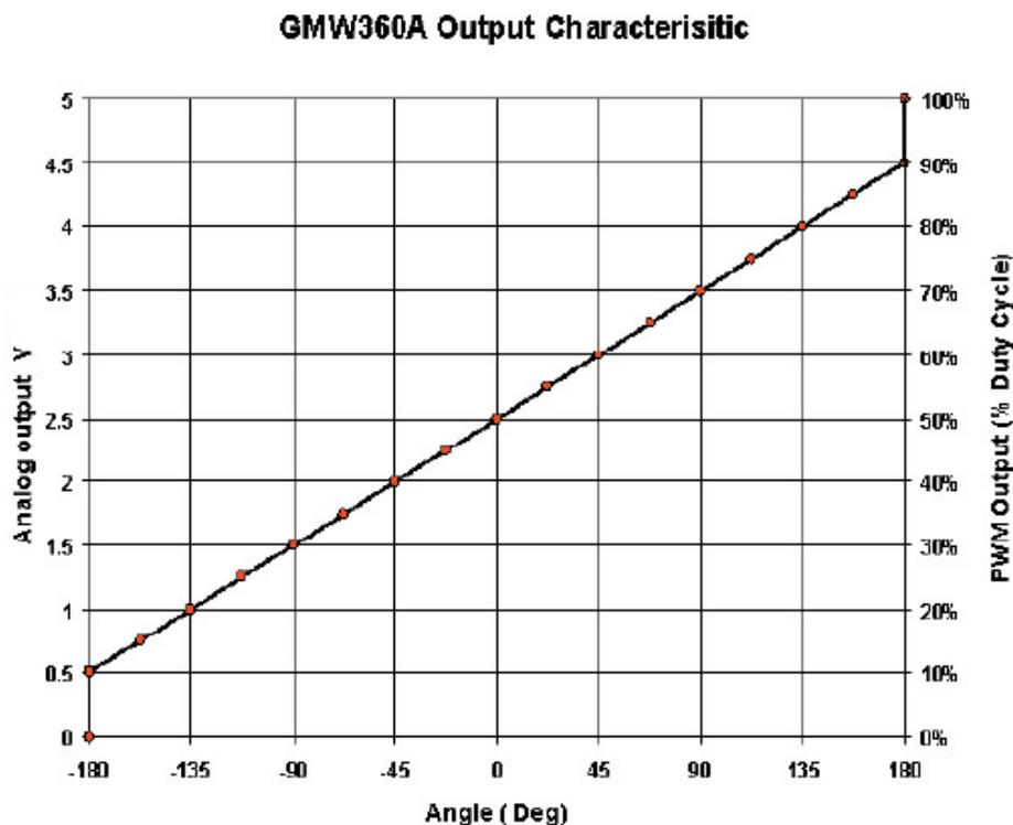
**Figure 19.** Output characteristic of the GMW360ASM.
