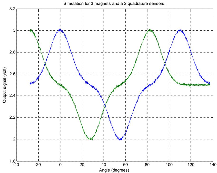
**Figure 10:** Simulation of the response of 2 sensor/3 magnet configuration.
